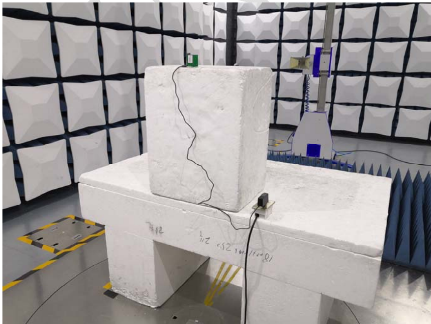
Radiated Spurious Emissions Test View (Above 1GHz)
